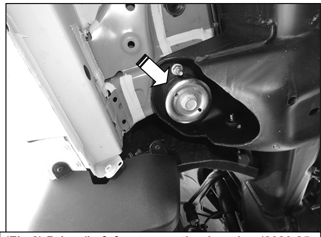
(Fig 2) Driver/Left front mounting location (2020 25-3500 model with cupped body bolt washer shown)
